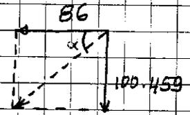
$$2. \quad a_{B/n} = \frac{v^2}{r} = \frac{(116)^2}{200} = 67.28 \text{ m/s}^2 \angle 30 \quad a_t = 2 \text{ m/s}^2 \angle 60$$
