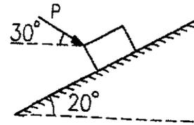
10% 1- Draw the free body diagram and the kinetic diagram of the package.
