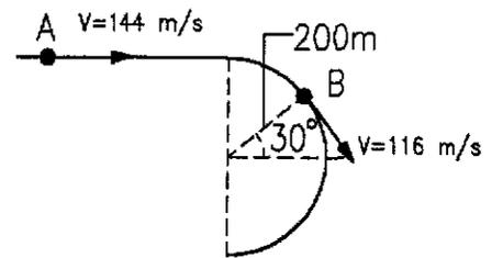
10% 1- Determine, for the position shown, the velocity of B relative to A.
